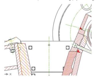
damage from excessive wear or impact. The deflector plate benefits from this wider angle, as it can better deflect oversized feed material, ensuring smooth operation. By protecting the bearings, which is a key component, this design improves the crusher's overall efficiency and longevity.
