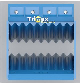
By evenly distributing pressure across the entire surface, the crusher can handle even the hardest materials with ease. This tooth-to-tooth configuration enhances grip on tough materials, allowing for better fracture and reduced wear, ultimately boosting performance and durability in demanding crushing applications.
