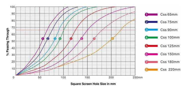
The product graph and the percentage of the crusher product that is smaller than the closed side setting (square hole, mm) is dependent on the crushability of the material, size distribution of the feed material, as well as other factors.
