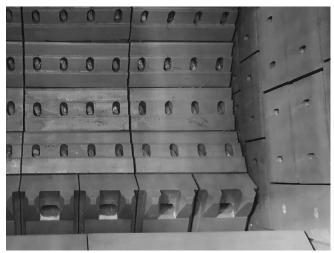
The standard modular impact plates and side liners are highly interchangeable within the crushing chamber, enabling maximum versatility. This results in higher utilization rates and longer service wear life.
