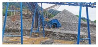
A steel tunnel was installed at the side of the existing primary stock pile. A total of 4 products were required. 0 - 50mm crusher run, 10 - 25mm aggregate product, 6 - 10mm chipping product and a 0 - 6mm dust product.
