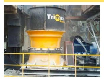
In late 2017, we were requested by a customer to give a proposal to upgrade his existing crushing plant. Through computer-aided simulation, we identified that the existing secondary cone crusher was the bottleneck. This led to a change to a larger Trimax NS400 Cone Crusher. We also identified that the existing final product vibrating screen would also need to be upgraded from a 2820 to a 2824 vibrating screen, in order to accommodate the eventual new total plant production.
