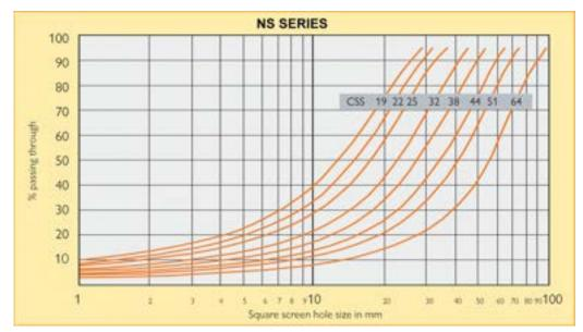
The product graph and the percentage of the crusher product that is smaller than the closed side setting (square hole, mm) is dependent on the crushability of the material, size distribution of the feed material, as well as other factors.
