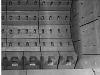
The standard modular impact plates and side liners are highly interchangeable within the crushing chamber, enabling maximum versatility. This results in higher utilisation rates and longer service wear life.
