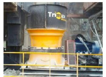
In late 2017, we were requested by a customer to give a proposal to upgrade his existing crushing plant. Through computer-aided simulation, we identified that the existing secondary cone crusher was the bottleneck. This led to a change to a larger Trimax NS400 Cone Crusher. We also identified that the existing final product vibrating screen would also need to be upgraded from a 2820 to a 2824 vibrating screen, in order to accommodate the eventual new total plant production.
