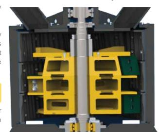
Feed material entering the crushing chamber from the This highly efficient method of crushing has relatively top is immediately met with the high centrifugal force low power requirements, and results in reduced
